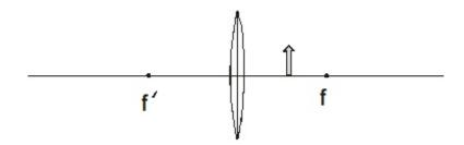
**10.** A double convex thin lens has a focal length of 35.0 cm. A 2.15 cm tall object is placed 10.0 cm from the lens, find (a) the type of image, (b) the image distance, (c) the magnification, (d) the image height.
